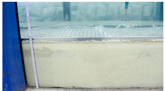
Fig. 6. The geotextiles and metal screens on the seabed surface.
