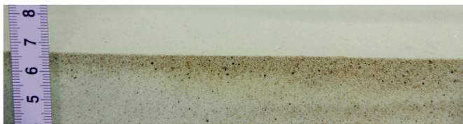
Fig. 9. Sheet flow with a height of 10–15 mm and the sorted grains on the bed (Case 5).
