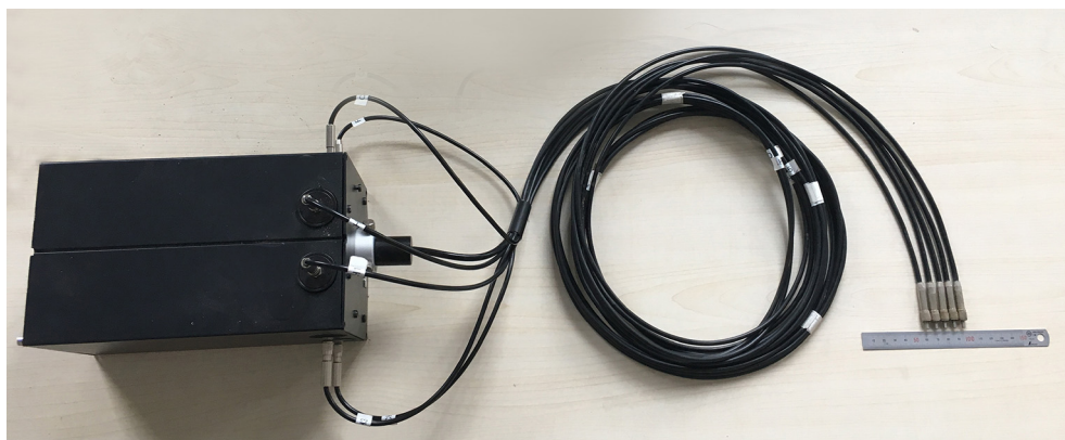
Fig. 3. Five-channel miniature optical fibre sediment concentration measuring instrument.
